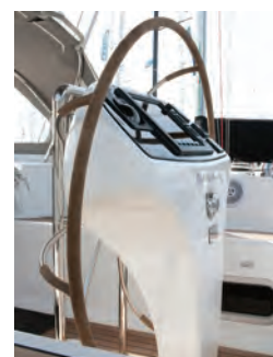
Custom dished wheel designed to mount on the back face of the customer's own pedestal for which they have a registered trademark.
