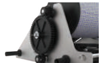
Heavy-duty gears transfer the power of the 400W integrated motor-gearbox via the main shaft to the feeder arm mechanism.
