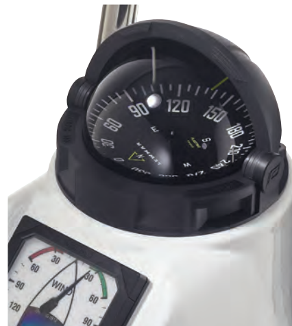
Lewmar 135 Compass flush mounted in pedestal
